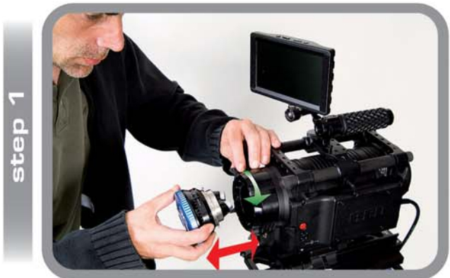
Adjusting of the 'FDC' to the camera. Switching-on of the 'FDC'.
